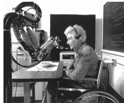
Fig. 2 Robotic Feeding System developed by Kawamura and others during the 1990s
